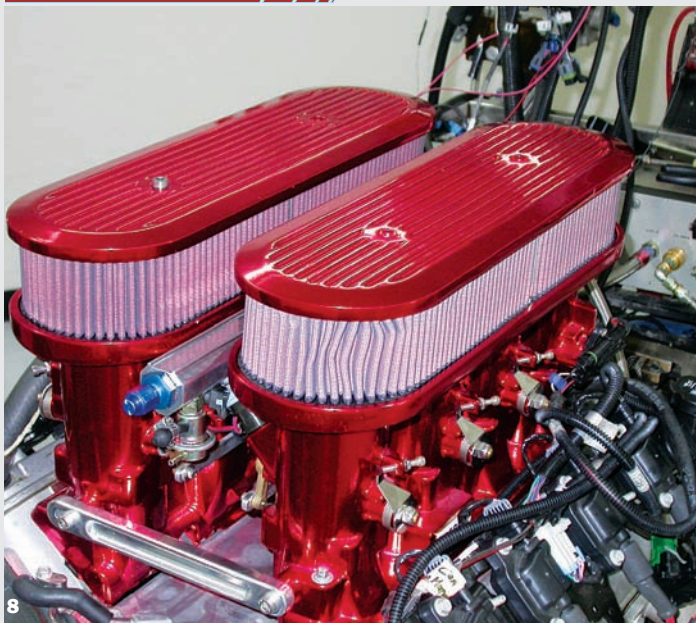
8 Off came the stock LS2 intake, and on went the Pantera EFI IR manifold. Talk about impressive-looking! 9 Running the same air/fuel ratio and timing, the IR manifold improved the peak power output from 463 hp and 450 lb-ft of torque to 486 hp and 456 lb-ft of torque. 10 We wondered if the air filter assemblies might represent a restriction, so we ran a test with the filters removed. There was no change in power, so make sure to run the filters on your classic Chevy.
