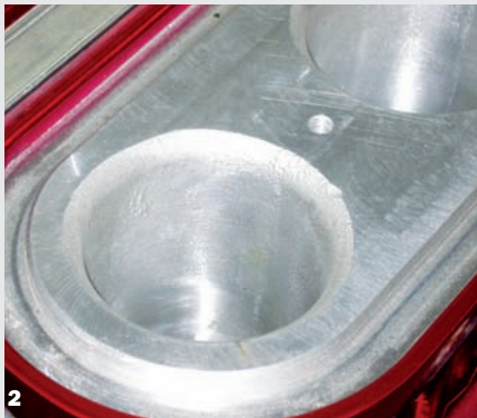
1 Each runner was equipped with a 2-1/2-inch butterfly to maximize flow to each runner. 2 To further improve power, the individual-runner intake also featured radiused air entries.
