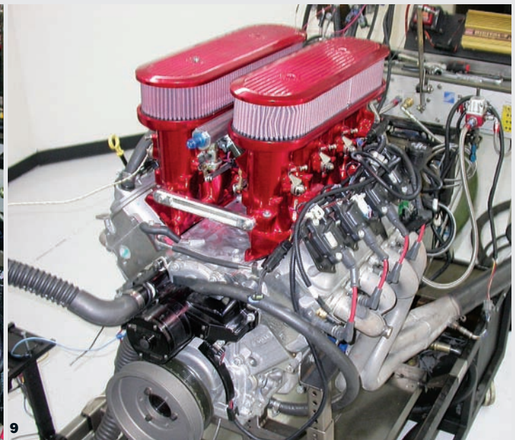
8 Off came the stock LS2 intake, and on went the Pantera EFI IR manifold. Talk about impressive-looking! 9 Running the same air/fuel ratio and timing, the IR manifold improved the peak power output from 463 hp and 450 lb-ft of torque to 486 hp and 456 lb-ft of torque. 10 We wondered if the air filter assemblies might represent a restriction, so we ran a test with the filters removed. There was no change in power, so make sure to run the filters on your classic Chevy.
