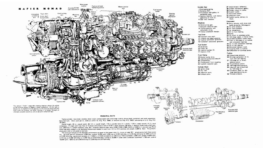
FIG. 11-12 Napier Nomad. The reader may consider this a complex engine, but Napier did not; for example, it described the flat-twelve two-stroke Diesel that formed its reciprocating component as "the simplest possible type." (Courtesy of Flight via NASM-Smithsonian.)
