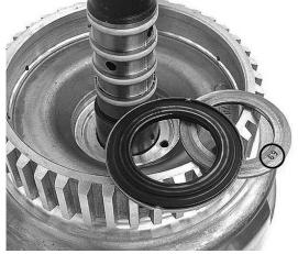
Once you know the correct selective washer size to use, install the correct selective washer under the thrust bearing on top of the input drum.
