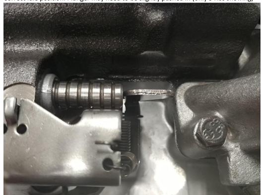
WOT plunger is pulled all the way into the plunger sleeve to its stop.
