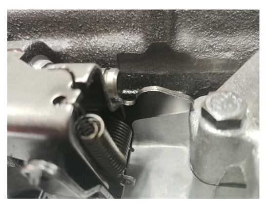
Correct Idle position. Plunger may need to be slightly pushed in (only 5 ribs showing)
