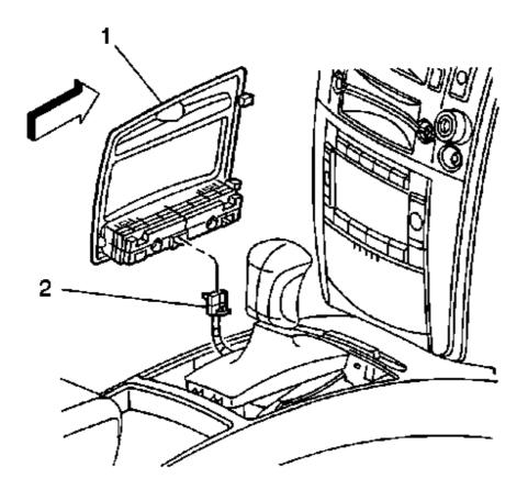
2. Disconnect the electrical connector (2) from the shifter trim cover (1).
