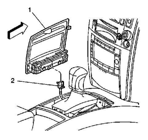
4. Install the shift indicator lamp electrical connector (2).
