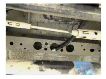
Tie strap the hose and vent assembly (referring to the graphic above, depending on the vehicle model). The CTS and STS should be strapped to the rear crossmember frame. The SRX should be strapped to the underbody sheet metal reinforcement.
