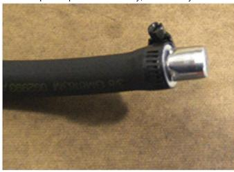
Assemble the new vent onto the hose and clamp the outer shoulder of the vent. Referring to the graphic above.
