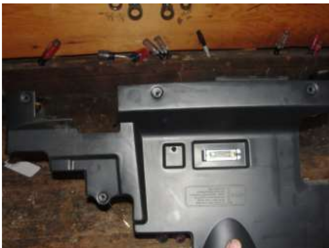
Small pic of the plastic cover off to show where the 4 screws are located
