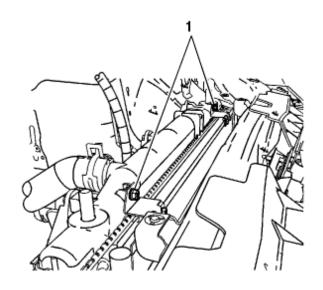
Notice: Refer to Fastener Notice in Service Precautions. Install the upper condenser mounting bolts (1). Tighten the bolts to 6.5 Nm (58 inch lbs.).
