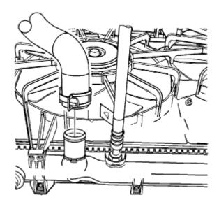
Using J 38185 disconnect the lower radiator hose from the radiator.
