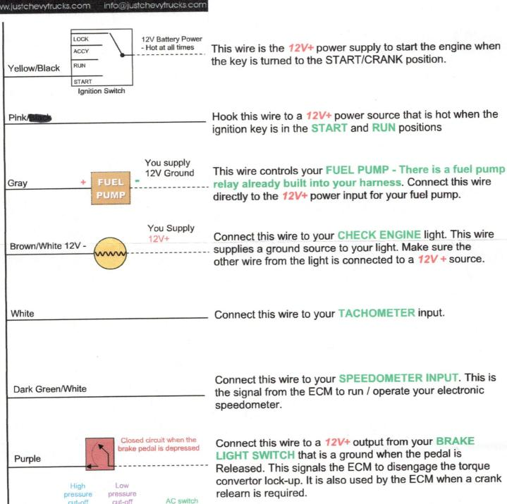
Connect a 12V+ source wire from your A/C dash control to this wire. This will activate your A/C COMPRESSOR CLUTCH. We recommend you wire this in conjunction with a relay and HIGH & LOW pressure cut-off switches.
