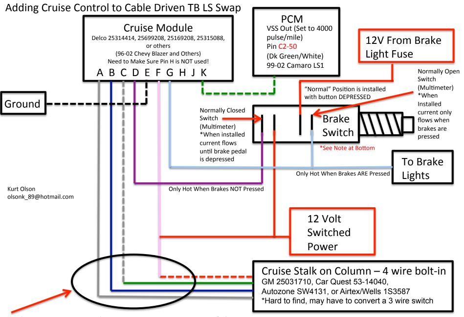
Gray (From Pin A on Cruise Module) – Goes to Gray on Cruise Stalk Switch = On/Off on cruise stalk
