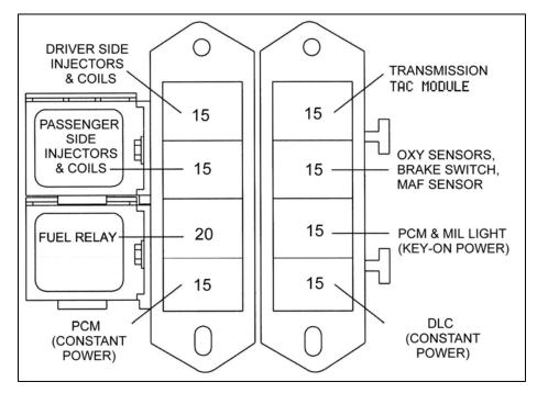
FIGURE 7.1 60522-23 Fuse Identification
