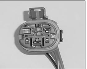
FIGURE 6.5 Fuel Pump Relay Connector
