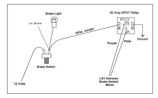
FIGURE 6.3 Brake Switch Relay
