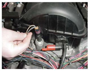
FIGURE 6.21 Oil Pressure Sensor
