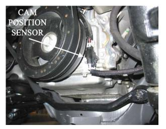
FIGURE 6.11 Cam Position Sensor
