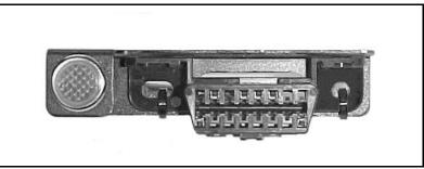
FIGURE 6.1 DLC Connector & Check Engine Light
