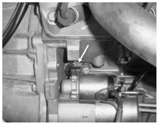
FIGURE 6.12 Crank Position Sensor
