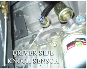
FIGURE 6.8 Knock Sensor Connector
