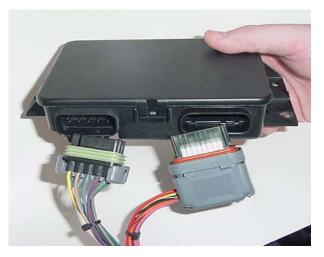
FIGURE 6.22 TAC Module Connections
