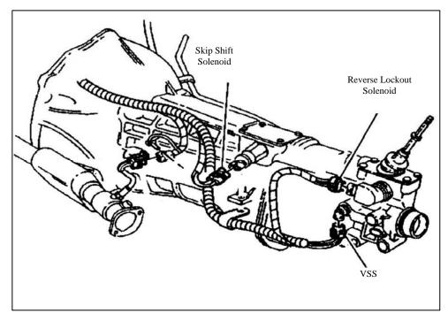
FIGURE 6.26 Transmission Connections (T56)
