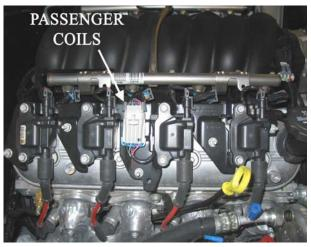
FIGURE 6.19 Passenger Side Coil Connector
