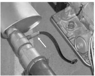
FIGURE 6.9 Oxygen Sensors
