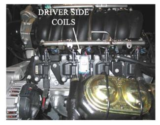
FIGURE 6.18 Driver Side Coil Connector
