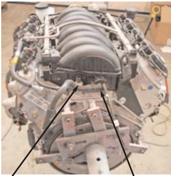
Stock oil pressure sensor Large vacuum port for power brakes and small port for accessories
