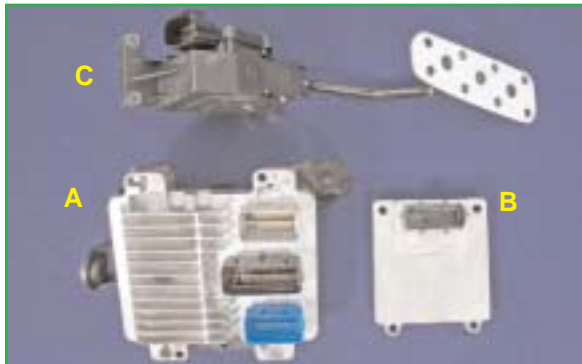
A. 05 LS2 Computer 12597883 B. Transmission Controller C. GTO DBW Throttle Pedal Assembly
