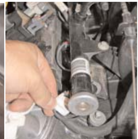
Connect the injector plugs to the injectors. The injector plugs are labeled driver side and passenger side.
