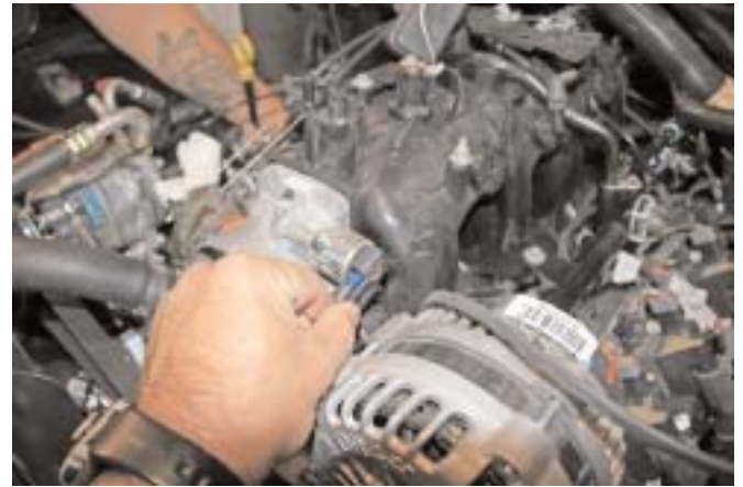
The idle speed motor is located at the top right side of the throttle body.
