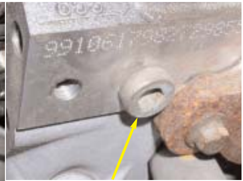
There is a water temp sensor in the front of the driver side head that is used by the engine computer. The 12mm plug located at the rear of the passenger side head can be removed to provide a locating point to install a sending unit for your coolant gauge (Factory, VDO ECT.) The head can be drilled and tapped for a pipe thread or S&P can provide you with a bushing to go from 12mm to either female 1/8, 1/4, 3/8 & 1/2 pipe.
