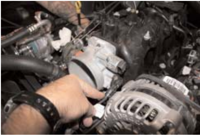
The throttle position sensor connection plugs into the bottom right side of the throttle body.
