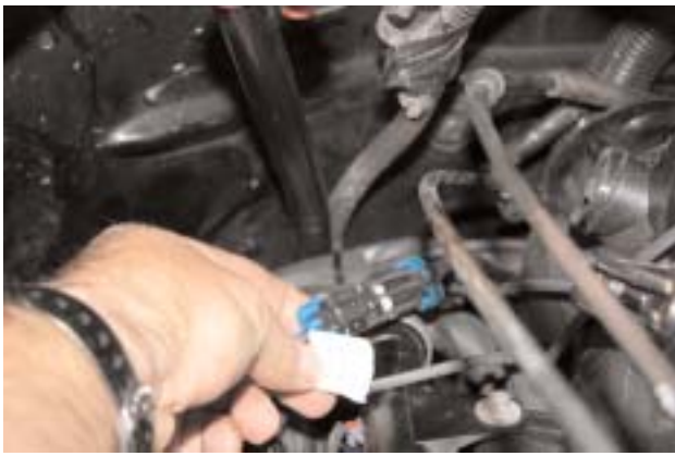
The knock sensor connection on the S&P harness connects to a pigtail that comes from under the back of the intake manifold.
