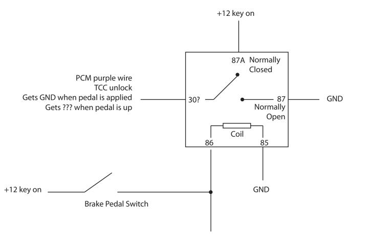
Light blue wire to Cruis Control brake input on TAC Get's +12 when pedal is applied, gets GND from coil when pedal is up
