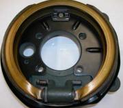
**3.** Emergency brake shoes need to be removed from the backing plate to provide clearance for the jet nut installation. Slide the brake shoes up to the very tip of the hold down spring.
