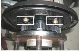
**10.** Reinstall the tappet and adjusting nut if the components were removed earlier otherwise detach the zip tie. Ensure pawl for <u>adjustment and the pin in the tappet are installed</u>.
