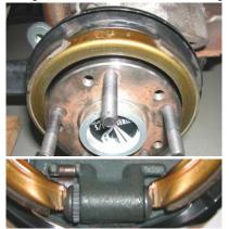
**12.** Pivot and push the shoes behind the hold down spring. Pull the shoes down to retain.
