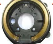
**4.** Pull the emergency brake shoes away from the backing plate to release from the hold down spring. Slide the shoes off the tappet and adjusting nut. Be careful not to move the lever in the back of the assembly otherwise the tappet and adjusting nut will slide out.
