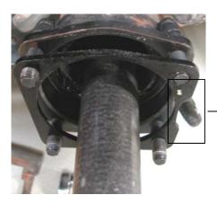
Ensure notch in spacer lines up with notch in housing end.
