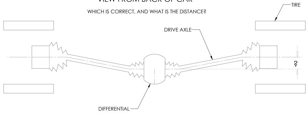
OR, ARE THE WHEELS CONCENTRIC WITH THE DIFFERENTIAL WHEN AT REST?
