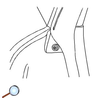
The weatherstrip in the area indicated shows where the weatherstrip relaxes and loses contact with the door glass. This generates windnoise. Refer to Figure 11.
