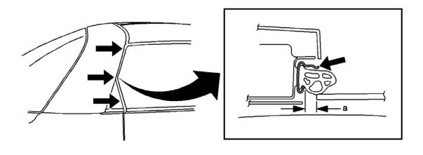
• Adjust the door glass forward or rearward to obtain a standard dimension of no more than 12 mm (1/2 in) from the edge of the glass to the retainer surface. Refer to measurement A in Figure 16.
