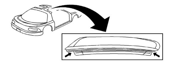
• The T-top rail weatherstrip is movable in the retainer and should be adjusted to only slight interference on the front and rear edges. The pressure of the closed glass will increase pressure on the joint once the glass is closed. Too much interference will cause the butt joint to pucker and provide a water path. Refer to Figure 13.
