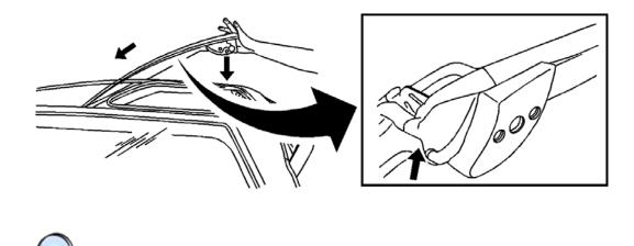
Make sure the customer is informed on the proper installation. Do not attempt to install the panels by sliding them horizontally toward the center roof rail. Doing so may cause the weatherstrip outer lip to fold under the removable top weatherstrip and may result in leaks and possible damage to the weatherstrip. Refer to Figure 14.
