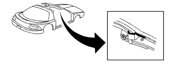
Apply a new seal using GM Silicone Sealant, P/N 12345739 (in Canada, use P/N 10953541), to the end of the roof gutter, under the molded weatherstrip detail, as shown in Figure 7.
