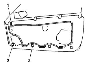
• Make sure the rectangular slot is taped over with duct tape. Refer to item 1 in Figure 2.
