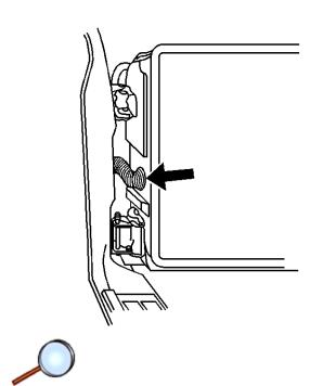
The door wiring harness rubber grommet may not be seated properly. Refer to Figure 10.
