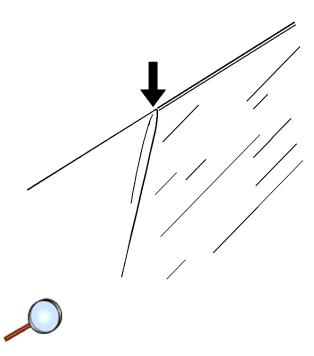
With the door open and the window up, apply pressure on the weatherstrip with a finger at the location shown by the arrow in Figure 20. The weatherstrip should not move.
