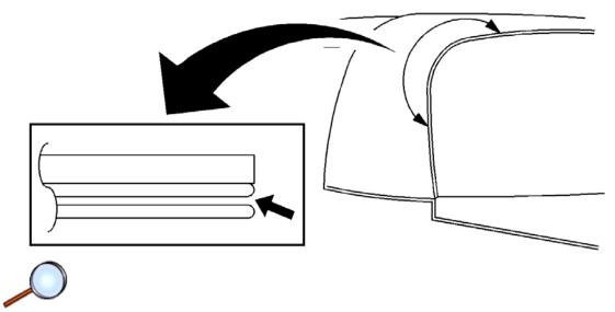
• Open the rear hatch to make sure there is no trapped water.
