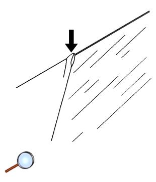
If the glass is not adjusted properly for height at the arrow, it will cause a bulge in the seal and create a windnoise. Refer to Figure 21.
