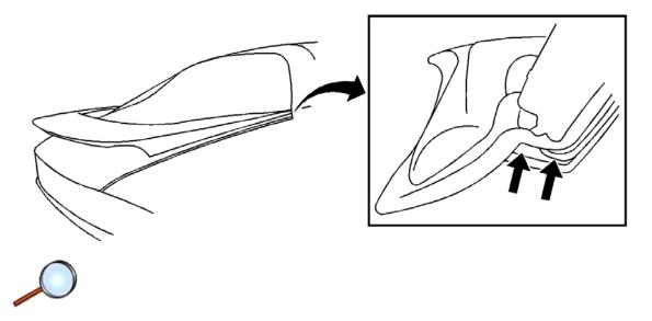
There is a water leak in the rear hatch (hard top, T-top models). Some customers may comment that when the rear hatch is opened, water runs out of one or both front lower corners. Refer to Figure 26.
