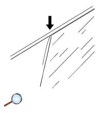
Align the mirror patch applique with the door open and the window up. The applique should be perfectly in line with the window or it should have a slight "bump" in the seal at the top of the mirror patch applique. Refer to Figure 19 for location.
