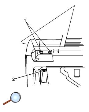
Adjust the window to the proper height to the roof weatherstrip. Then adjust the mirror patch to fit the door glass and the "A" pillar. Refer to item 1 in Figure 31 for up down and for and aft adjust. Refer to item 2 in Figure 31 for in and out adjustment.
