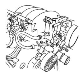
11. Install the PCV hose to the valley cover and intake manifold.
