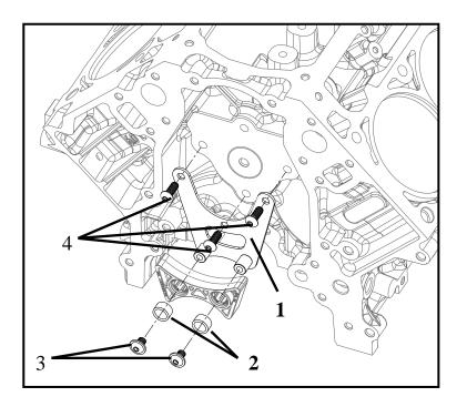
4. Place the timing chain dampener on the bushings on the adapter plate (should be a press fit) and place the aluminum spacers (if applicable) and the (2) M8 x 1.25 x 10mm flange bolts into the adapter plate bushing . Torque to 15-18 ft-lbs.
