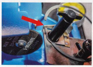
Serving double duty, this steel plate (arrow) squares the ring with the cutting wheel and provides a stop to keep the table from pivoting into the abrasive wheel. The knurled knob on the right is adjustable and once set, makes squaring virtually automatic. We didn't touch it after the first ring. Once the ring is square and touching the squaring plate, it is held in place by tightening the wing nut on the taller post.
