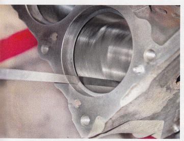
[Taking 0.005 inch at a time, we crept up on the 0.0019-inch gap of the top ring. Don't force the feeler gauge in place; we found out that 0.0017-inch feeler gauge would fit just right, but a 0.0019-inch feeler gauge could be crammed in the same gap.
