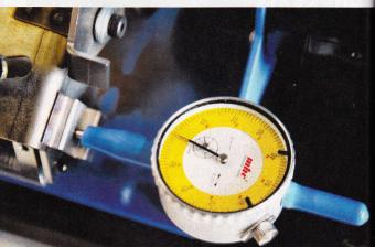
With the motor off and the plate rotated out of the way to allow the table to pivot, we turned the knob on the left of the table to drive the ring toward the abrasive wheel while holding the table down. As soon as we felt contact between the ring and the wheel, we stopped turning and set the dial indicator to zero.
