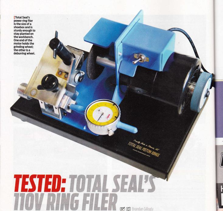
> Few processes in assembling an engine are as tedious as filing piston rings. It requires patience and precision, carefully fitting the top and middle rings to each bore. It's not something for an assembly line. Considering the new ring packages used in modern pistons often include thin but tough steel or ductile iron rings that make old cast-iron rings seem soft in comparison, the thought of using our old hand-cranked ring filer gets less and less appealing. That's where
