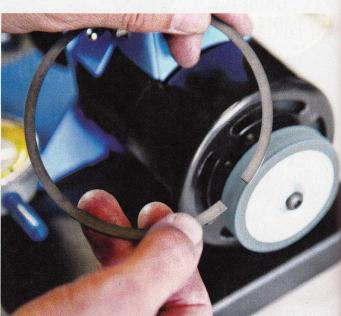
[Before the rings are considered done, they must be deburred. A very light touch is all it took to knock off any accumulated metal with the fine-grit wheel opposite the gap-filing table. This can also be accomplished with a razor blade, as the burr tends to be holding on by the narrowest of threads.
