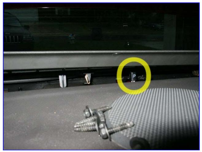
12. Remove the HUD. The HUD is held in place by 1 screw, 2 bolts and the electrical connector. Remove the bolts on either side of the HUD, remove the screw from the area behind the instrument panel, unfasten the wire connectors on the side (passenger side of the HUD), then lift the HUD out of the dash. I had to slide it out towards the passenger side. Once out, I took it to my work bench (kitchen counter top :-).
