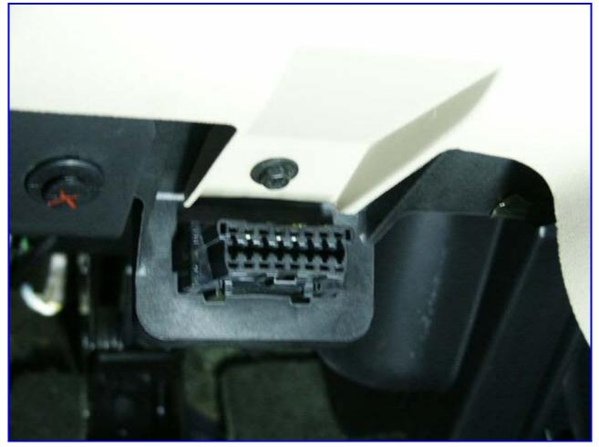
7. Remove the knee panel (lower dash panel). Remove the 2 screws at the bottom and 1 on the left side. Once the 3 screws are out, you can pull it away from the dash. It has a few guides at the top that hold the top in place.
