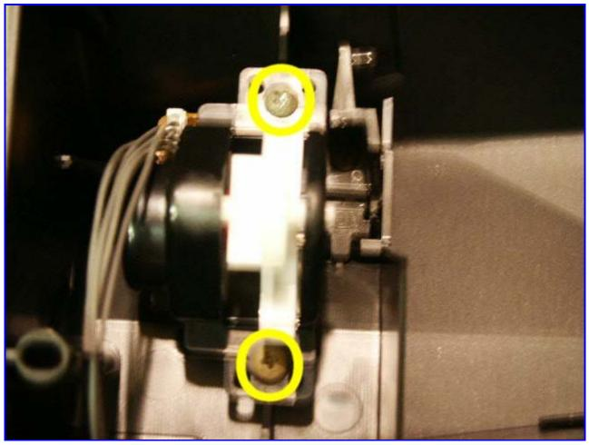
17. Drill a hole in the bracket. I drilled the hole just right of where the spring pulled through the plastic (see photo). I guess someone could use epoxy of something to fix the split but why chance it.
