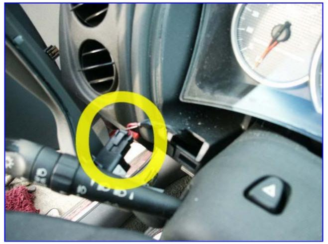
9. Remove the instrument cluster. It has 4 screws that hold it in place. Remove the screws, pull it a little away from the dash, un-fasten the wire connector that connects to the cluster, then lift it away from the dash.
