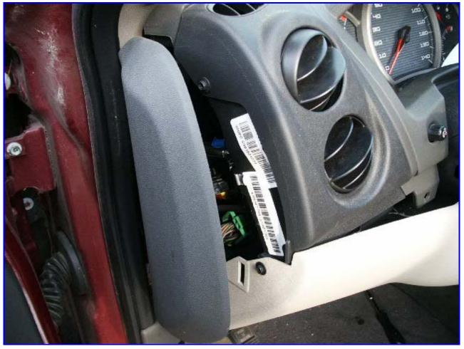
6. Un-secure the OBD-II connector. Look under the dash near the center area of the drivers side, you will see the OBD-II connector. It has a clip securing it in place. Take the clip loose and push the connector back a little so you can get the screw above it out.
