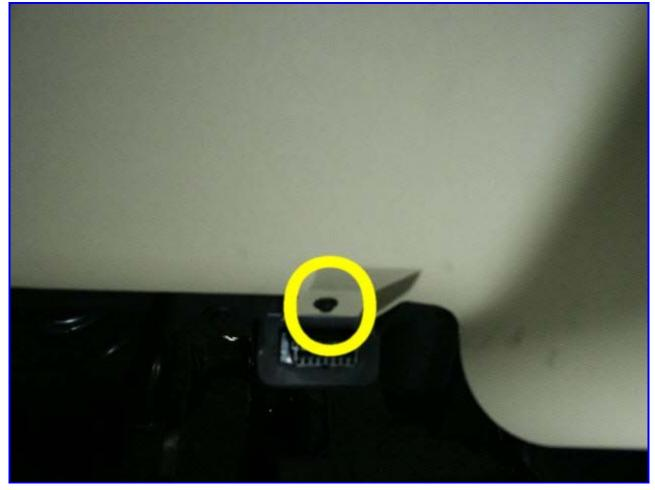
8. Remove the panel that goes around the instrument cluster. It does not have any screws holding it in place, just 3 clips at the top. I pulled at the top to get it loose, removed the wire that connected the light dimmer, then lowered the steering wheel and lifted the panel away from the dash. NOTE: Be careful not to break the wires that connects to the dimmer knob.
