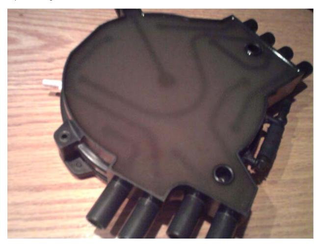
When installing the cap & rotor to the distributor body, a lot of folks have noted it's a good idea to lay a bead of RTV along the top seams between distributor body and isolator, and even a little bit between isolator and cap. Be careful and use your best judgement.
