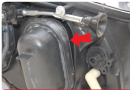
High beam cover loose
