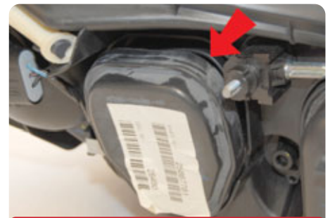
Low beam cover loose
