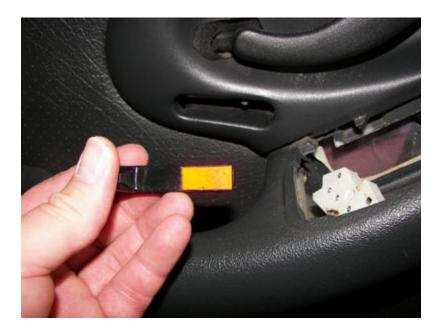
With one hand raise door handle and with the other move the cover in the direction of the arrow to release the light in the cover:
