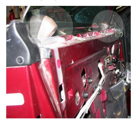
You will have to remove the plastic water protector, not shown. Mine was already coming off, but if yours is stuck, try to use a hair dryer to heat the glue to remove and install it back properly.
