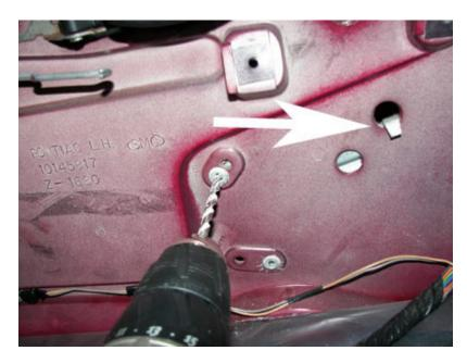
Move front door rear window guide channel out of the why of the motor assembly wheels and channels. Try and pull the entire motor and assembly towards the rear access hole. You will need to get the assembly wheels out of the guide channels. Once you do, you will be able to remove the assembly out of the rear access hole. The big hole is the access hole, but trusts me; the whole is not nearly big enough. You will have to pull them out of their channel guides.
