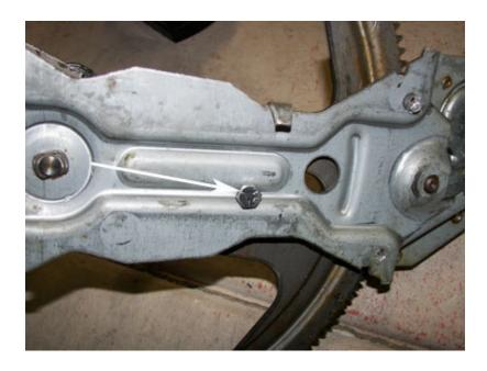
With the assembly secured, you can now safely remove the motor. You have to drill out the three rivets:
