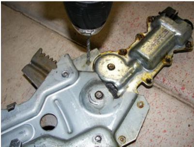
Once you are done with the three rivets, the motor will fall off:
