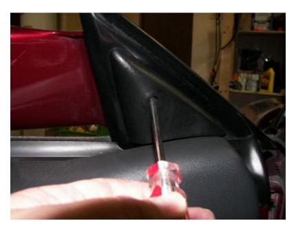
Pull it straight out from the door, being careful to not break the small retainers:
