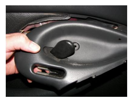
Now you will have to disconnect the light. To remove the light, grab the connector and twist it. It should come off with ease:
