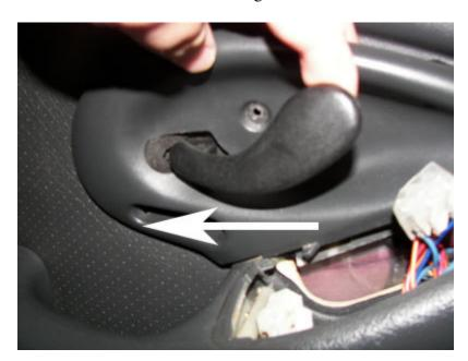
With the cover loose, raise the handle and maneuver the cover off the door handle:
