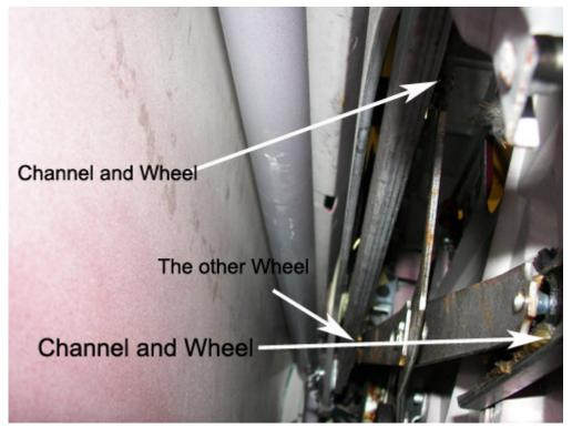
Now you will have to remove this from the rear access hole. The manual shows it as a small assembly, but here is what will emerge:
