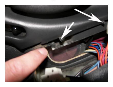
Next pull off the two connectors, and use a screwdriver for the center one. Use one hand to move the clip lock and the other to pull the plug off:
