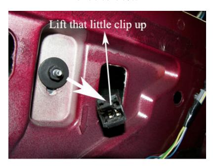
You can easily remove the plug by going through the speaker hole:
