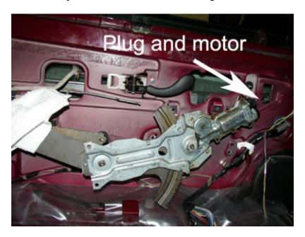
Here is a photo of the plug and a photo of where it connects to the motor. I pulled it out of the door so you can see it and how it connects to the motor. You cannot see in this area, so you have to go by feel and it's quite a clumsy process. I also think the plug is different on the 97.
