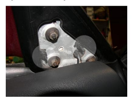
Next, remove the 4 screws holding the door panel to the door with a LARGE Phillips screw driver:
