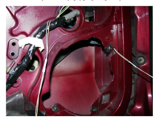
Now it's time to find the four rivets you will need to punch out and remove.
