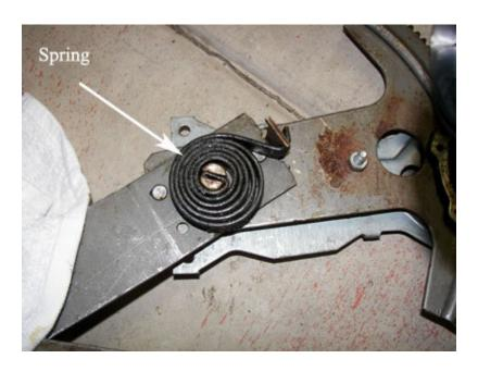
As you can see in the photo above, the assembly is under tension, so you must now drill a hole and place a bolt in that hole to keep it secured and from spinning around and causing injury. Drill the hole:
