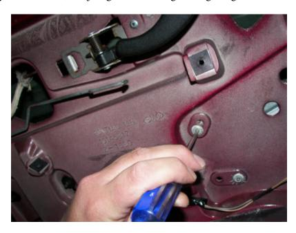
Drill the rivet heads completely off. You don't need to go all the way through the door. Pay special attention to the hook in the photo below. You will know when you have completely drilled out the rivets because that hook will become very loose. Remove the hook from the door and lay the motor on the bottom of the door.
