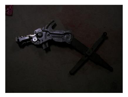
It's not difficult to remove, but you do have to move it around and mess with it to get it out. You have to pull it towards the access hole. And, the motor (the silver part) is towards the door hinges or front of the car, so you won't see that right away. You have to get the little wheels out of the guides. That takes a little time, but 20 minutes for me on the first time.
