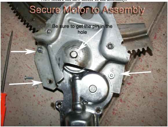
With the motor secured, you can now remove the bolt you had installed to secure the sector gear. Be careful and make sure to stay clear in case the gear moves, but it shouldn't:
