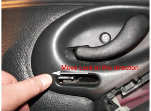
Now grab and pull the lock slider over the handle cover as shown below:
