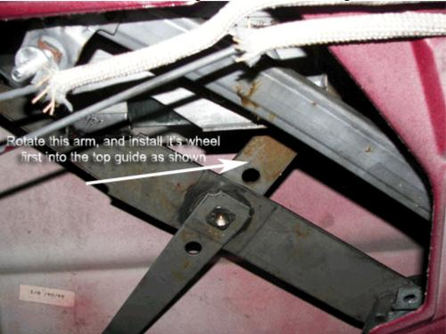
Now get #2 into the same guide. You will have to push to motor towards the front of the car to make the wheel travel in its guide and to get #2 into the guide.
