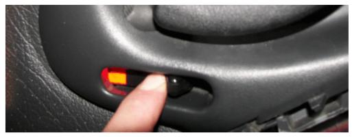
Tighten down the handle cover. Grab the switch panel, connect the connector and press the panel straight down onto the door panel:
