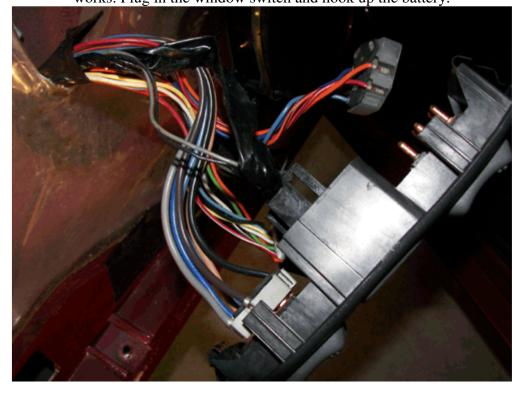
Turn the ignition key to the "ON" position and see if the window motor works. If it works, this would be a good time to grease up the channel guides and wheels. Raise or lower the window until you see the guides and wheels and grease them up:
