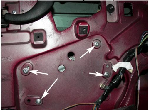
Tighten down the front side door window rear guide channel:
