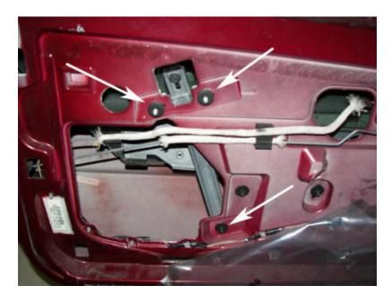
Now reach through the same speaker whole and put the plug back onto the motor. After the motor plug is attached, you may need to move the window up or down **manually** in order to get the holes for the rivets to line up. Make sure the motor does not fall off when you are doing this. You can use a couple of small screw drivers to make sure the doles
