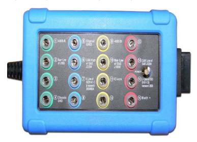
The CAN Test Box (CTB) is a diagnostic tool which connects to a vehicle's OBDII connector and is used to easily diagnose electrical faults.
