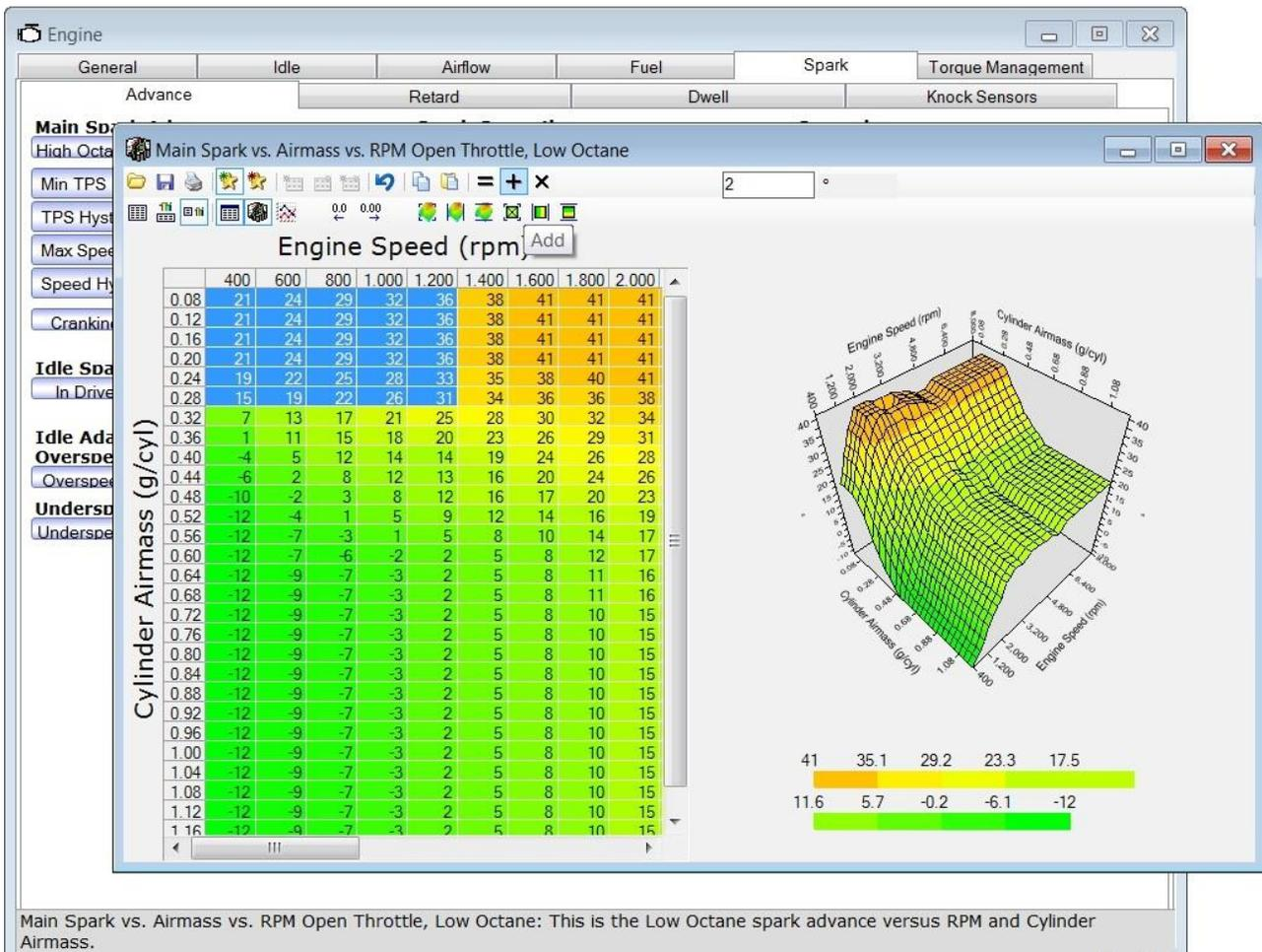
Cams with over 0° overlap up to 15°, idle 900-950 all cells across the board, add 2 g/sec to idle airflow across the board both in P/N and in gear (**HPT > Engine > Idle > Idle Airflow > Base Running Airflow**), add 4° of idle timing 1200 RPM and under and 0.08 – 0.28 g/cyl inclusive (**HPT > Engine > Spark Control > Spark Advance > Idle Spark Advance (in Park)**).
