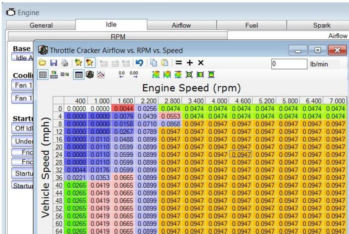
Throttle Follower parameters do not need too much adjustment IMHO. I kept them stock (from a 03 SS file) however did bump up the decay values (doubled) in the 0-4 MPH cells in all gears so that my idle would come to rest a little quicker with less fluctuation.
