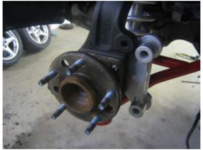
Image 2- Drivers side bracket installed with hub
